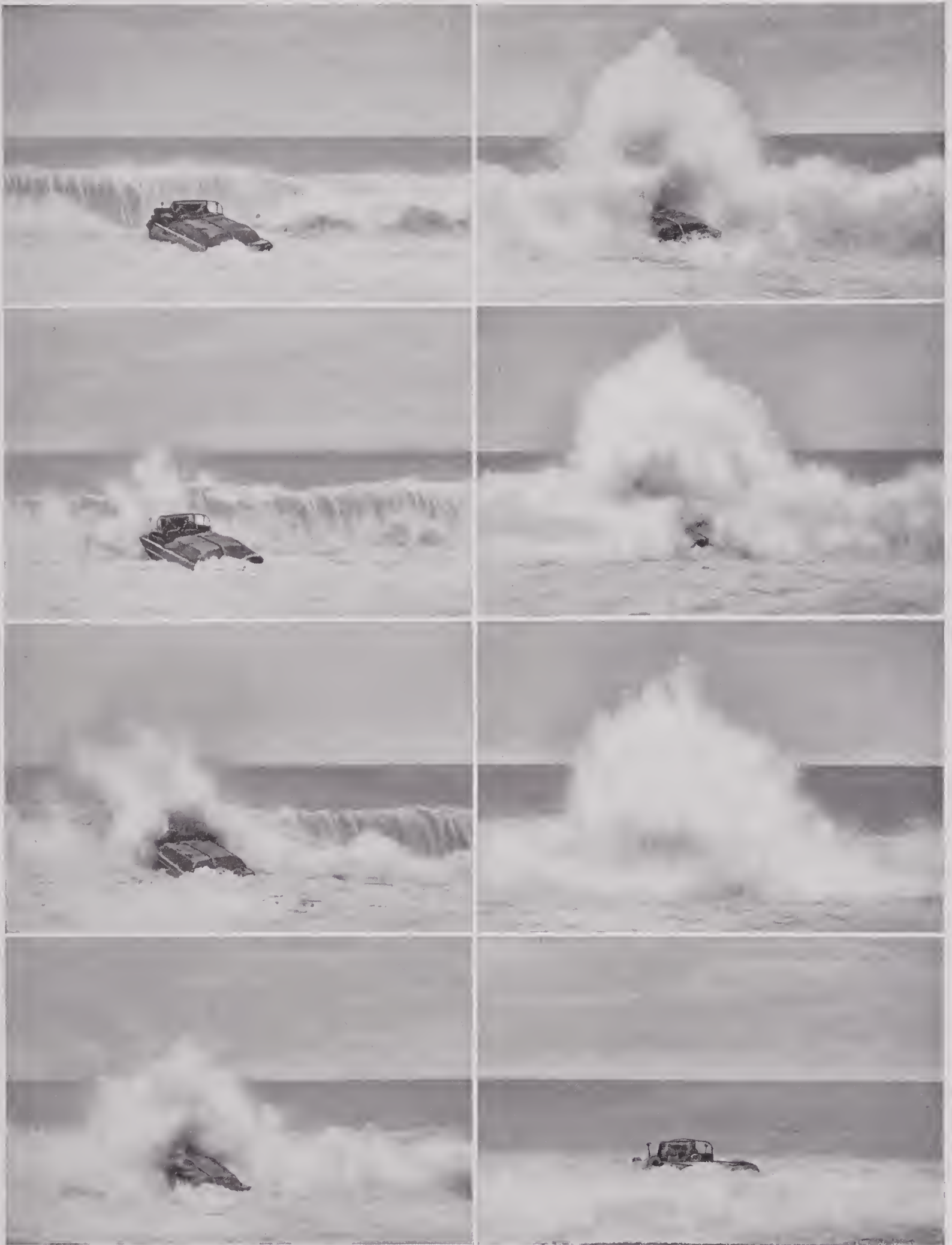
FIGURE 53. Series of photographs showing laden DUKW standing out through solid afterbreak of 15-foot comber on steep-to beach at Monterey Bay, California. Course is deliberately somewhat diagonal and is unaltered. Speed is temporarily reduced from about 4 knots to about 1 knot.
